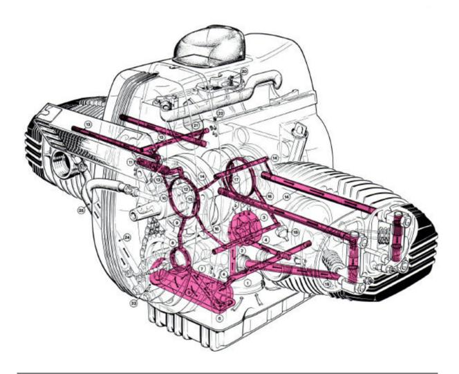
There are three other oil takeoffs at the front mainbearing cap. One applies oil pressure to a spring-loaded pressure relief valve (11) which limits oil pressure to a maximum of 74 psi at high rpm. Another feeds the oil-pressure pickup sensor (18) and then the rear mainbearing. The third is a drilled oil gallery (15) in the crankshaft itself which feeds the lower-end bearing of the left connecting rod. A similar gallery (17) from the rear main bearing feeds the right lower-end bearing.
